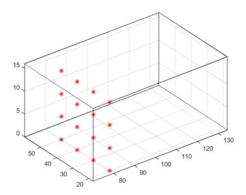
You do not need to use 3-D arrays, such as those returned by meshgrid, but the size of each array must be the same, and meshgrid provides a convenient way to generate arrays when you do not have an equal number of unique values in each coordinate. You can also define starting-point arrays as column vectors. For example, meshgrid returns 3-D arrays:
