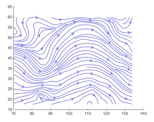
This stream slice plot indicates that the flow is in the positive x-direction and also enables you to select starting points in both x and y. You could create similar plots that slice the volume in the x-z plane or the y-z plane to gain further insight into your data's range and orientation.
