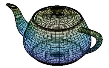
If the FaceColor property is set to 'none', then the object appears as a wire frame diagram. p.FaceColor = 'none'; % turn off the colors
