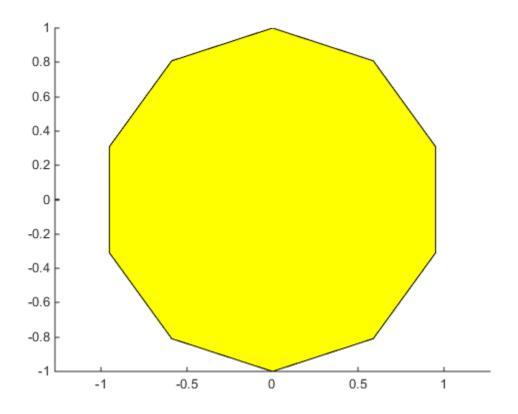
The first and last vertices need not coincide; MATLAB automatically closes each polygonal face of the patch. In fact, it is generally better to define each vertex only once, particularly if you are using interpolated face coloring.
